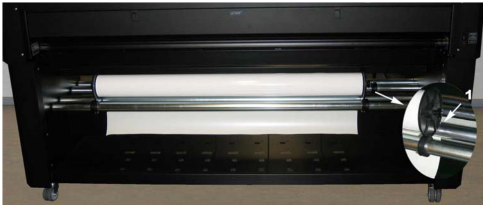
FIG 1-11 POSITION OF THE SUPPLY ROLL ON THE DC4
