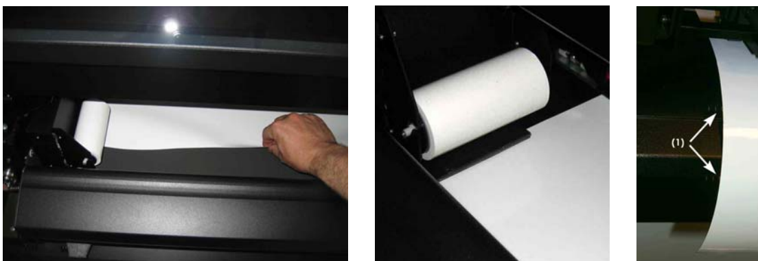
FIG 1-13 LOADING ROLL AT THE FRONT OF THE DC4
