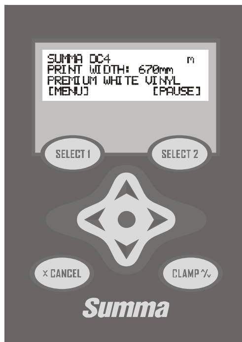
FIG 2-1 DC4 CONTROL PANEL
