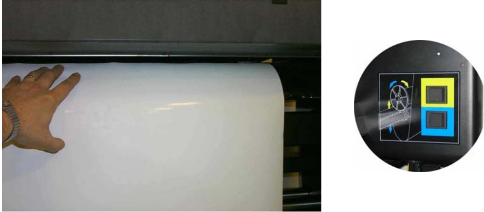
FIG 1-12 LOADING ROLL AT THE BACK OF DC4
