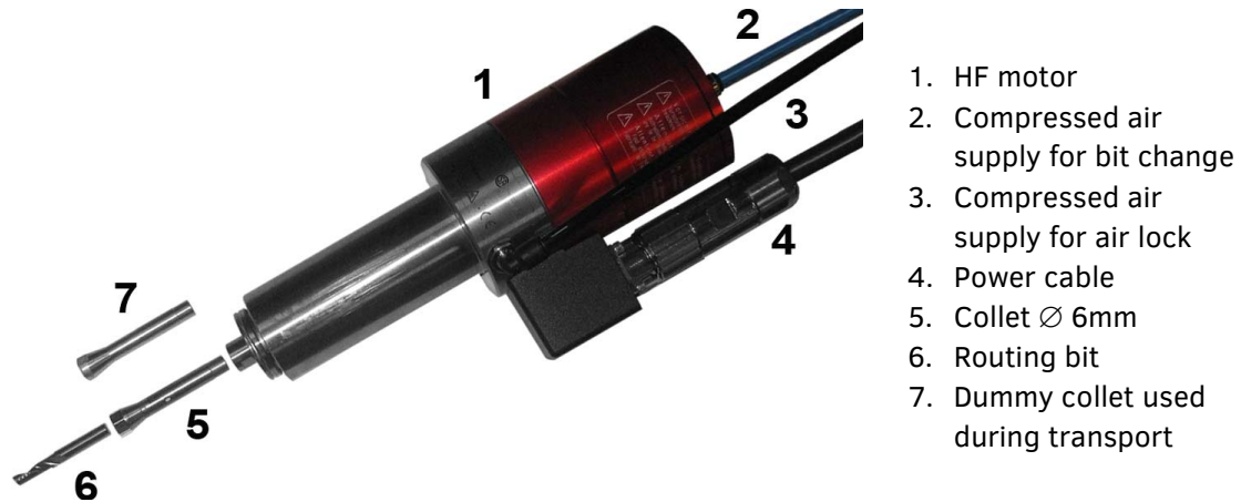
FIG 2-28 HF MILLING MOTOR
