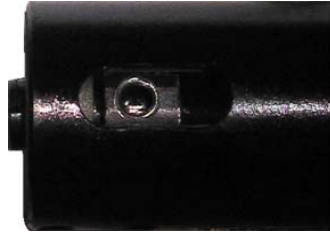
FIG 1-30 KNIFE HOLDER SHAFT – SETSCREW REMOVED FROM EOT
