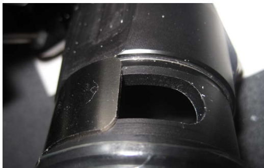
FIG 2-82 RING TO SET THE VACUUM STRENGTH
