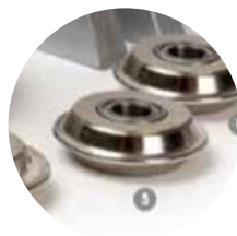
5 Scoring tool: 32 mm diameter, 1.5 mm round crest.
