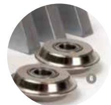
6 Scoring tool: 32 mm diameter, 1 mm round crest.
