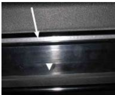
FIG 5-3 SLIDING SURFACES ON Y=GUIDE RAIL
