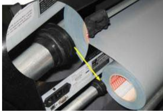
FIG 1-19 FEEDING ROLL MEDIA WITHOUT USING THE FLANGES
