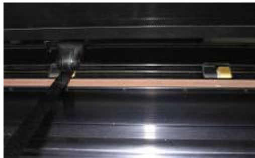
FIG 5-1 PLACEMENT OF VINYL STRIP
