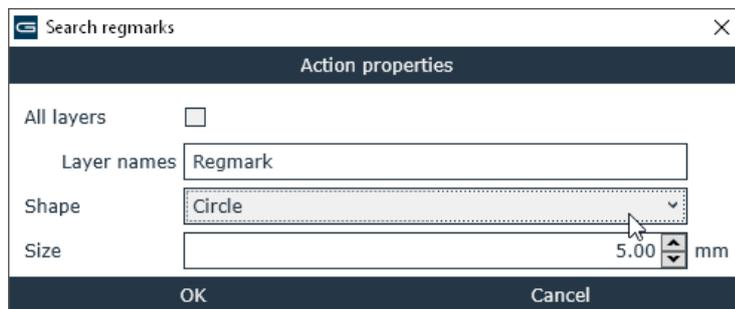
You have the option to scan all the layers or to fill in the name of a specific layer. Also, the shape and size of the registration mark can be set. Set all the parameters to the desired value and click the OK button. Then click the search regmarks icon. If there are any registration marks on the chosen layer, they will get the
