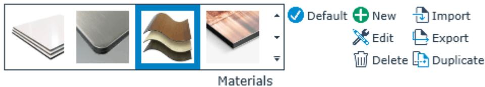
The different materials are categorized into groups to facilitate retrieving the needed material. Click the drop-down arrow at the right side of the materials' pictures to scroll through the categories. Then select the material. The selected material has a blue contour around it. Materials can be added or deleted, edited or set as default.
