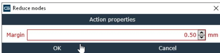
Right-click the reduce nodes icon to set the maximum distance, used to delete a node. The maximum value is 0.5 mm.
