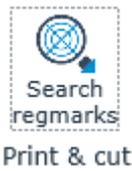
This function will search the registration marks on certain layers. Normally, the registration marks are recognized while importing the file. However, in some cases, extra registration marks on special layers may have been added or the file, which needs to be imported was not correctly prepared. In this case, this function can be used to scan each layer for registration marks. First, click right on the icon. A window will open with the settings.
