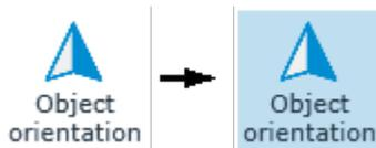
Use this to reveal the orientation of the object. Click it and a triangle will be shown at the start point of each object, showing the direction of the curve. Click the triangle to reverse the direction, if necessary.
