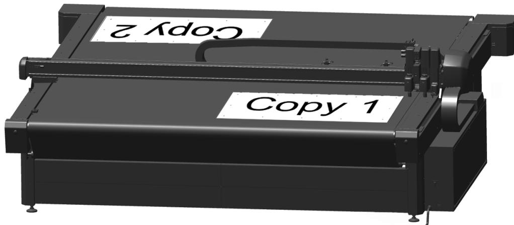
In order to facilitate loading the jobs on the table, it is recommended to mark the place where the media has to be loaded. It is not necessary to do this each time the tandem mode is used. Only when the lines are faded, is it necessary to redraw them.
